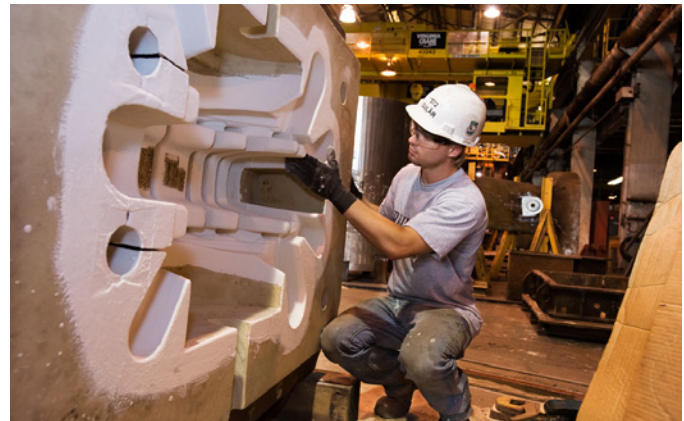
Newport News Shipbuilding Foundry Apprentice Daniel Gular sands the surface of a mold for a gate valve. The gate valve was used in the refueling and complex overhaul of the aircraft carrier USS Theodore Roosevelt (CVN 71). Photo courtesy of Huntington Ingalls Industries.
