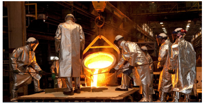
Newport News Shipbuilding apprentices pour molten steel into a mold in the shipyard's foundry. Photo courtesy of Huntington Ingalls Industries.
